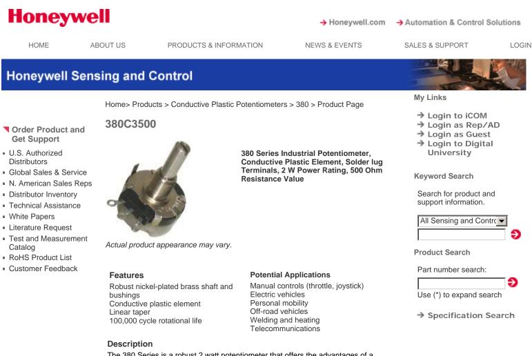
The 380 Series is a robust 2 watt potentiometer that offers the advantages of a conductive plastic element and a 100,000 cycle rotational life. Special tapers and element designs available on a special order.
